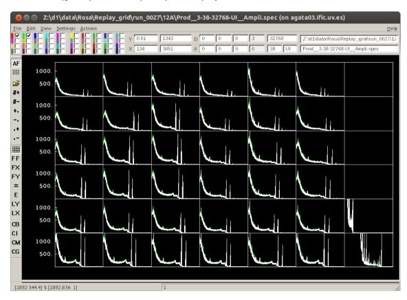
12A Core Prod\_\_3-38-32768\_\_Ampli.spec [0][36] online data (green) and after (white) the Replay on GRID run 27
