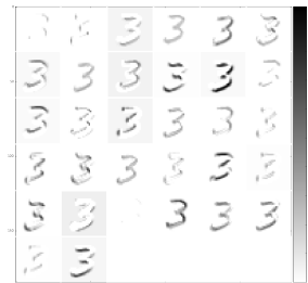
Outputs of first Convolutional layer for above input
