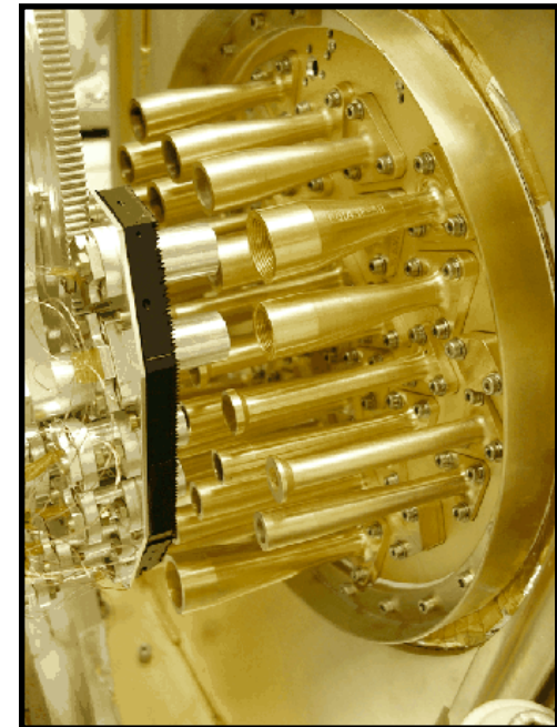
HFI focal plane & calibration sources
