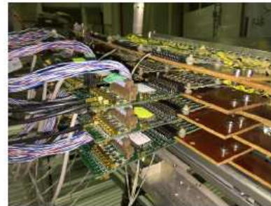
Front-end electronic cards with PASTTREC ASIC.
