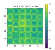
Figure 49: Efficiency map of one photodetection module of the EUSO-SPB2 mission, developed, integrated and calibrated in the photodetection laboratory
