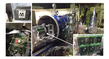
Figure 95: Top left: Dose tests with a Cobalt 60 source at COCASE (CEA Saclay). Bottom left: SEL tests with a Californium 252 source at TRAD (Toulouse). Right: SEL qualification at the cyclotron of UCL Louvain (Belgium)
