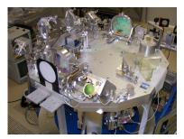
Figure 97: One of the Virgo modematching telescopes delivered by APC
