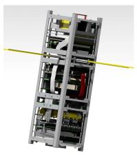
Figure 44: 3D view of the integrated satellite (without its solar panels)
