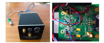
Figure 18: Fibered high frequency photodiodes needed for the new Advanced Virgo control scheme, which uses auxiliary green laser beams
