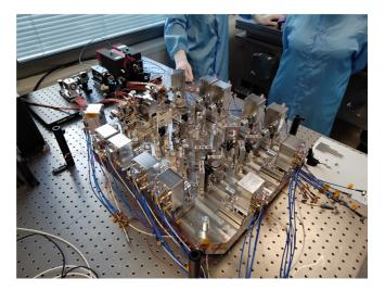
Figure 26 shows the MIFO bench in the final stages of optical integration (using an optical centering bench and a three-dimensional measuring machine).
