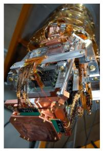
Figure 12: The dilution fridge in the millimetric wavelength laboratory
