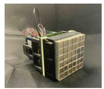
Figure 48: Assembled photodetection module for the EUSO-SPB2 mission
