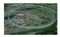
Figure 77: Illustration of the potential location of the Future Circular Collider at CERN, near Geneva. Also shown are the CERN PS, SPS and LHC rings, which would be part of the FCC injection and acceleration chain
