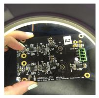
Figure 67: DUNE's SiPM analog transmitter
