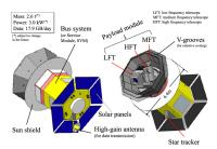
Figure 11: Conceptual design of the Lite-BIRD spacecraft. The payload module (PLM) houses the low-frequency telescope (LFT), the medium-frequency telescope (MFT), and the high-frequency telescope (HFT). From Hazumi et al. 2021 derivation of calibration requirements. The team is also expert in the modeling, characterization and removal of galactic foregrounds, which are the main limitation to the detection of primordial gravitational waves;
