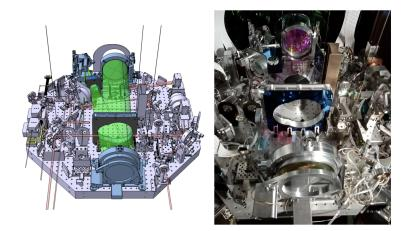
Figure 17: Global view of the optical bench at the detection port of Advanced Virgo (CAD design on the left and a picture on the right). The absorbing baffles designed by the team to mitigate stray light impinging on the optical components of the beamreducing telescope are evidenced.
