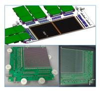
Figure 39: Bottom right: Photo of the Double Sided Stripped Detector, delivered in 2016. Left: its symmetric delivered in 2019. Top: Those two detectors are assembled to compose a half quadrant as shown in the sketch
