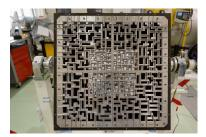
Figure 41: Picture of the flight model of the coded mask mounted on the ECLAIRs telescope. The shadow of the mask is reflected at the bottom of the camera by the detection plane
