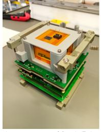
Figure 46: Prototype of the scintillation payload onboard IGOSat
