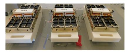
Figure 37: View of the three XGRE sensors flight models delivered to CNES in 2020
