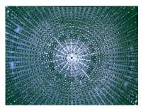
Figure 71: View of the internal of the Borexino Stainless Steel Sphere with PMTs (Credits: Borexino)
