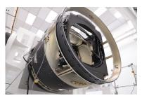
Figure 2: Picture of the assembled LSST camera under testing. One can catch a glimpse of the filter exchange system with the dummy filters inside – IR2 clean room – SLAC, California – December 2019. Credit: Gaëlle Shifrin, CNRS/IN2P3
