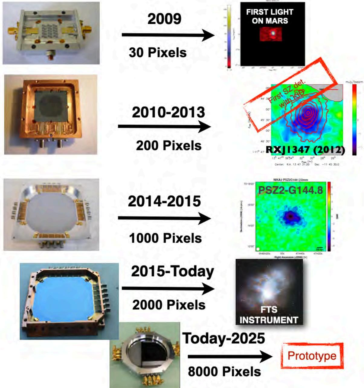
*Fig.1: KID array development during the last 14 years. From the first 30-pixel prototype of 2009 which has observed a first light at IRAM 30m telescope through the 200 pixels NIKA1 array which has performed the first observation of the Sunyaev-Zel'dovich effect with KID, up to the last 10k-pixels prototype fabricated and tested in our lab.*
