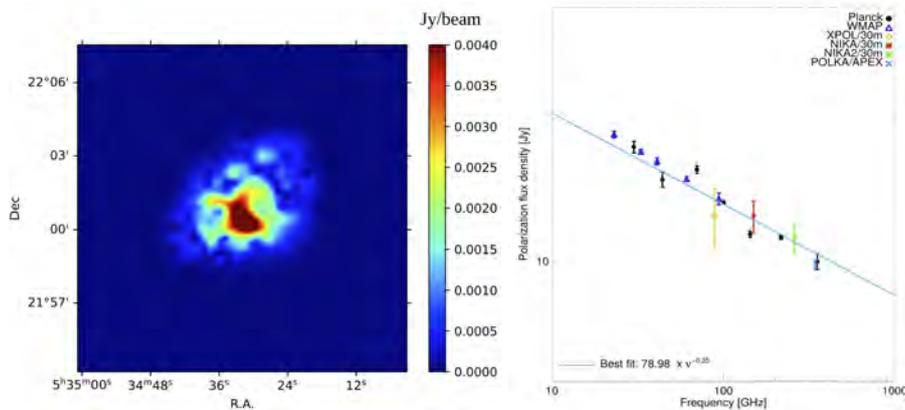
FIGURE 1 – Left : NIKA2 polarized intensity map of the Crab nebula obtained from NIKA2 observation at 260 GHz during the commissioning campaign of November 2020. Right : spectral energy distribution obtained by previous measurements accounting for the new value obtained from NIKA2 (green). Figure from [Ritacco et al. \(2022\)](#)
