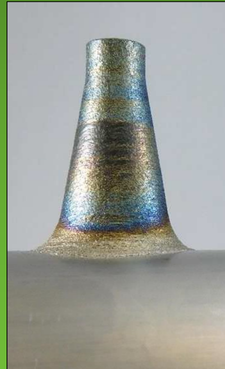
Addition on tubes in Inconel 625
