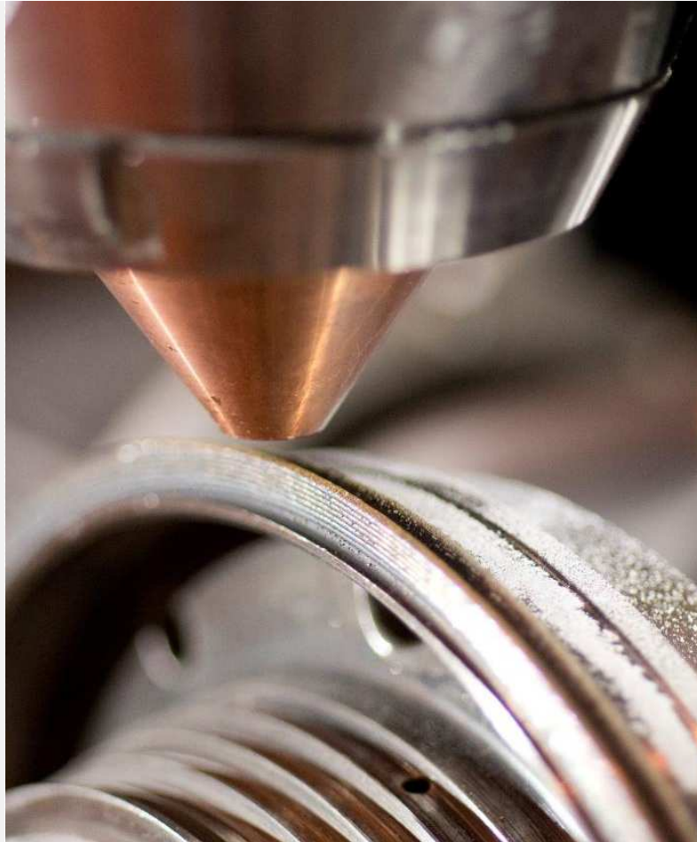
Worn shaft seal in Ti6.4
