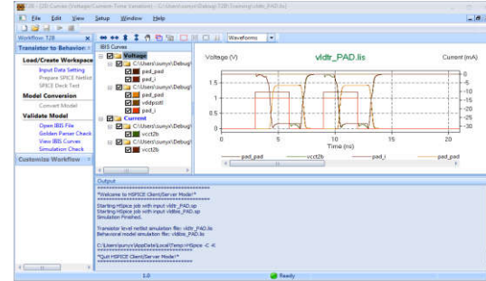
Built-in simulation check compares transistor to IBIS
