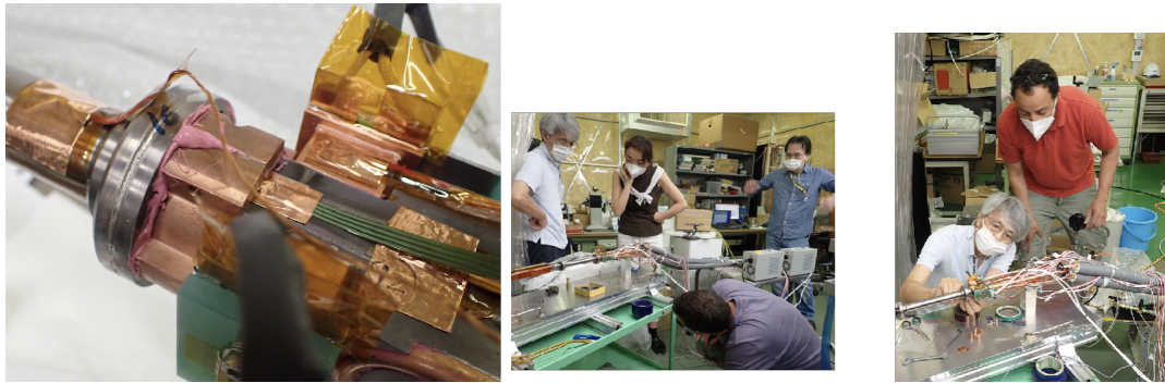
Figure 10: The new cooling block designed by IJCLab, (center & right) the final thermal test in collaboration between KEK/IJCLab engineers/researchers, July 2022 at KEK.
