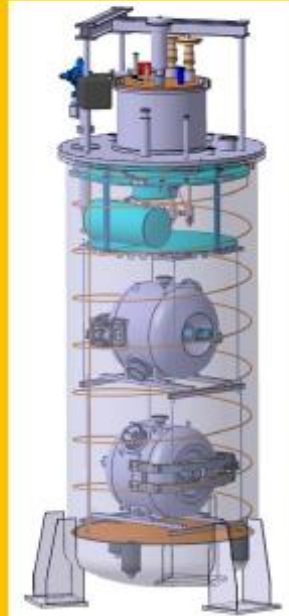
RF validation in vertical cryostat of 33 cavities + dedicated tuner
