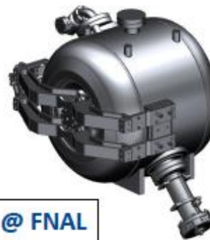
RF validation in horizontal cryostat
