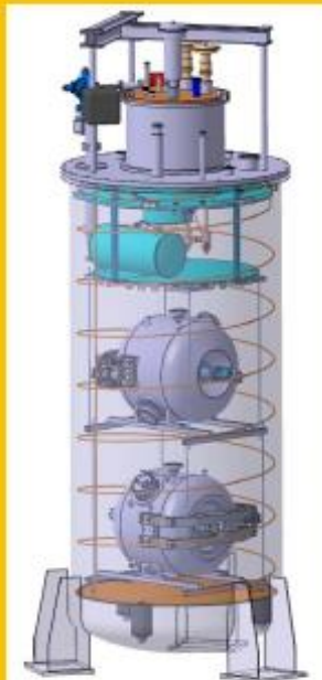
RF validation in vertical cryostat of 4 cavities
