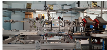
Fig. 14: BioALTO beamline under installation
