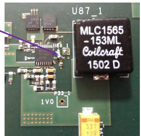
Figure 5: 1,5 k Ohms resistor, and 0603 package added.
