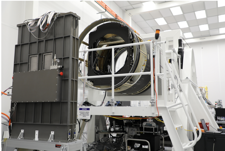
Filter exchange system during its integration in LSST camera at SLAC (Jan. 2020)
