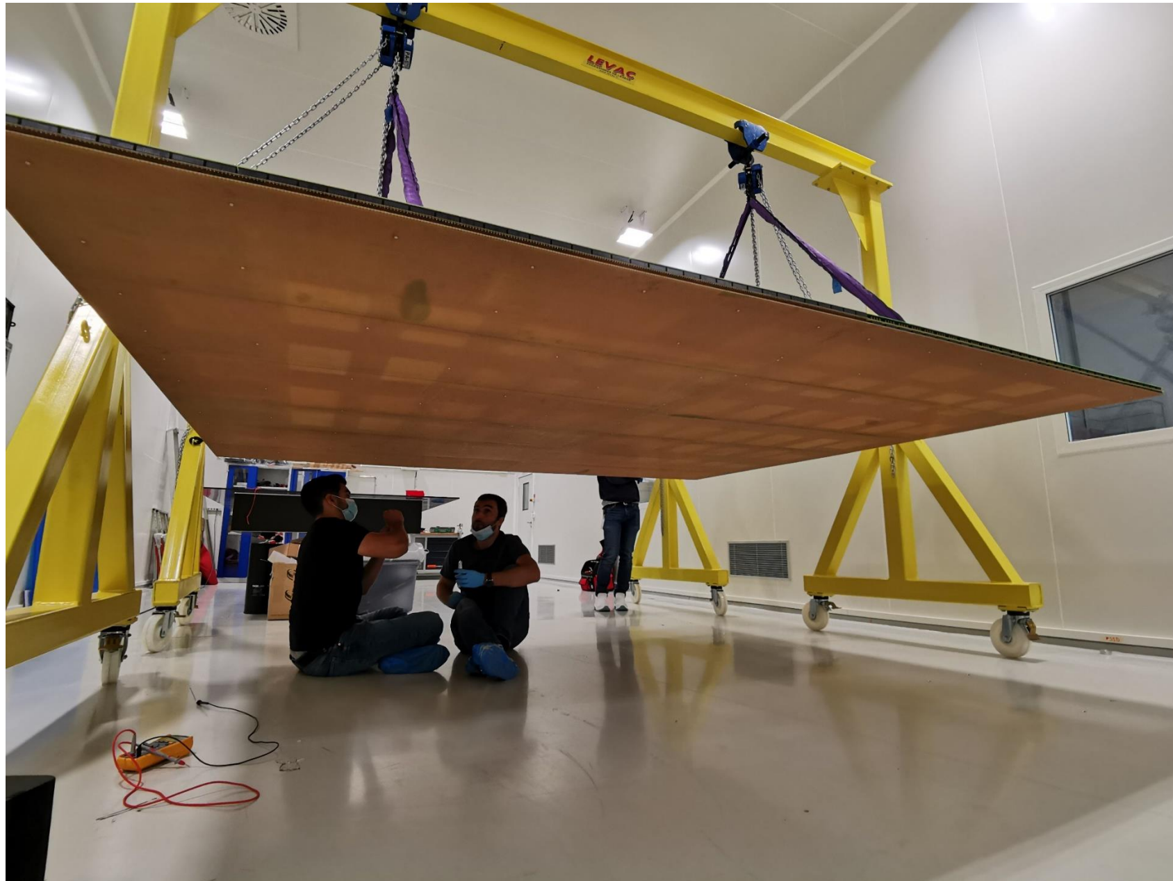
Fully assembled CRP seen from below
