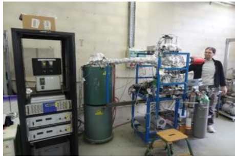
Figure 2: Set-up for Magnetron sputtering deposition.
