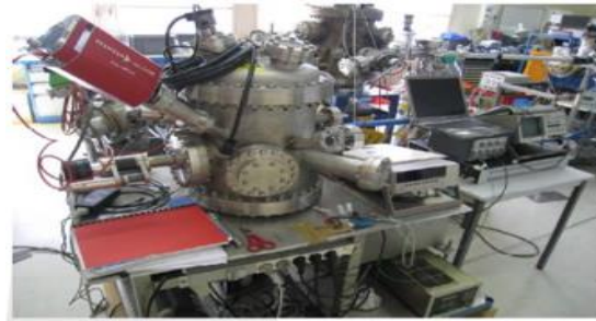
Figure 3: The experimental set up for secondary electron yield (SEY) measurements.
