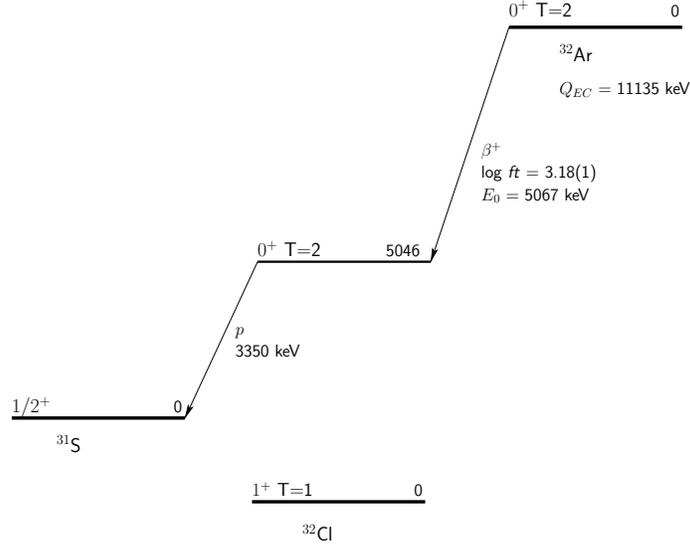
Figure 2: Part of the decay radiation scheme of the super-allowed  $0^+ \rightarrow 0^+$  beta decay of  $^{32}\text{Ar}$  (branching ratio 23%) to the IAS in  $^{32}\text{Cl}$  which then decays to the  $^{31}\text{S}$  ground state via the emission of a 3353 keV proton.
