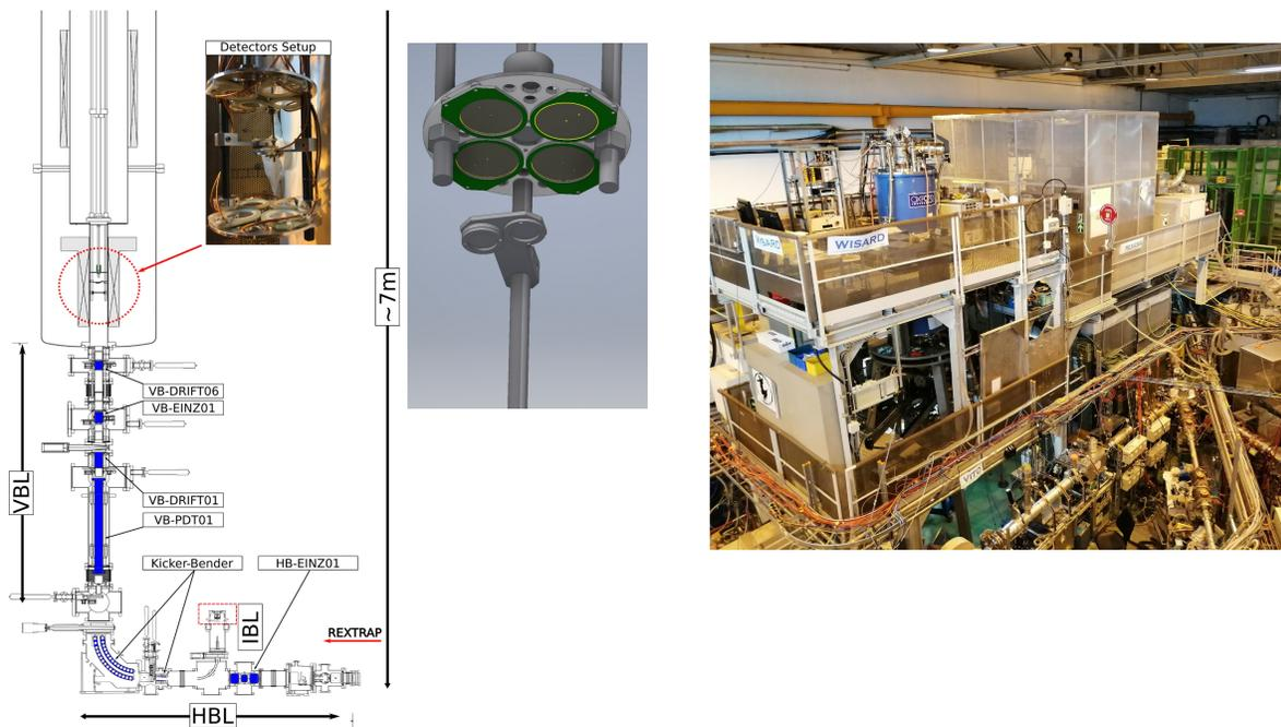
Figure 5: Schematics of the WISArD beam lines and of the proof-of-principle detection set-up, picture of the WISArD platform at ISOLDE.
