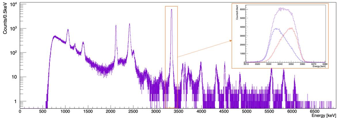
Figure 7: Total  $p$  spectrum in 1 strip closest to the beam axis of one DOWN detector. (violet : singles  $p$  events; red :  $\beta$ - $p$  coincidence events; blue :  $p$  events without  $\beta$  in coincidence)
