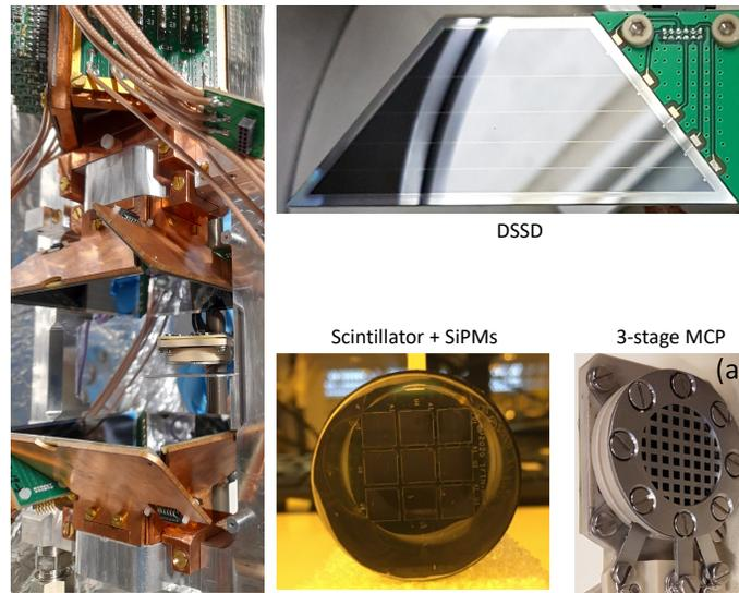
Figure 6: Pictures of the WISArD detection set-up with close-ups on 1 DSSD, the  $\beta$  detector and the triple-stage MCP.
