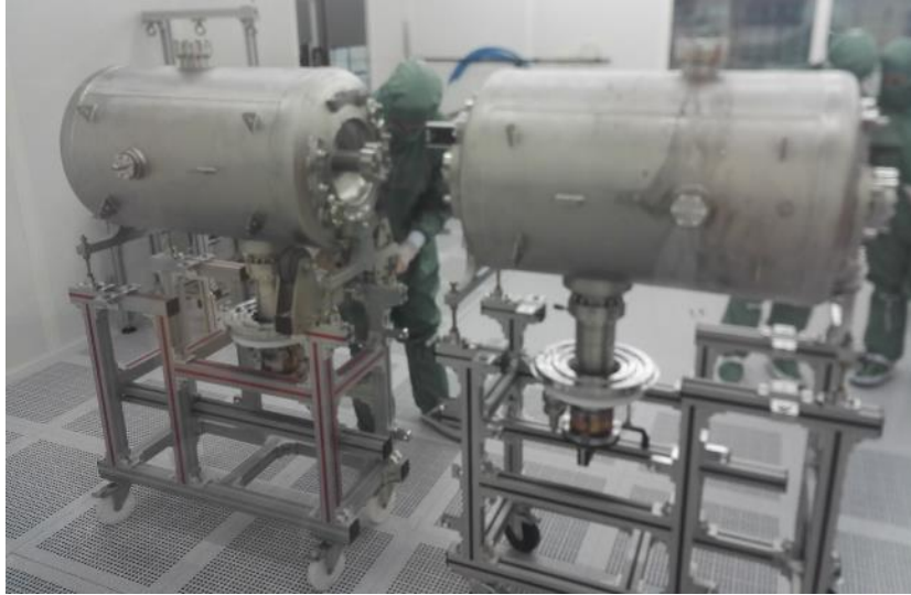
Figure 199 : Picture of a cavity string (2 cavities + 2 couplers) assembled together into the clean room at IJCLab.
