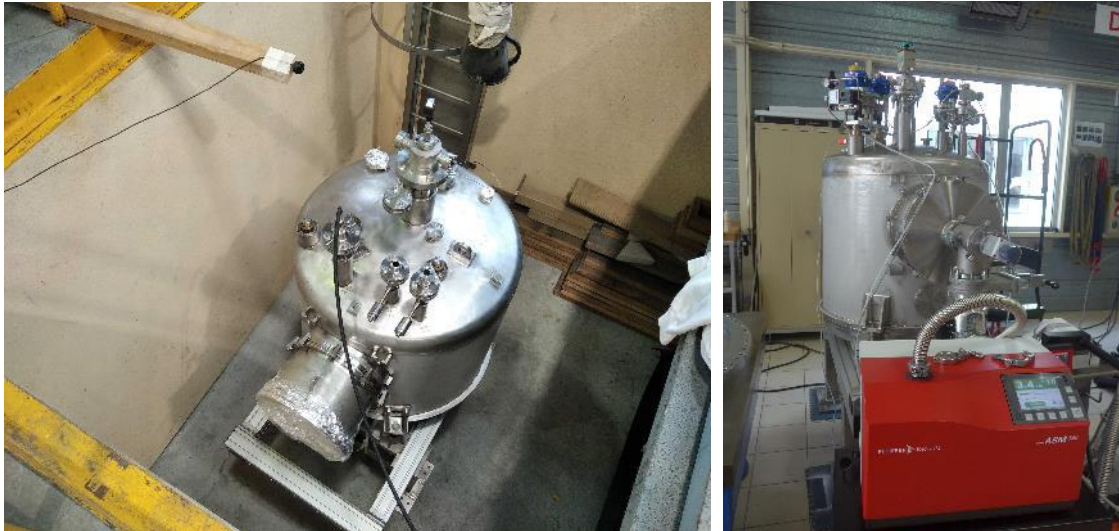
Figure 22: Picture of the End Box: Left: pressure test at SDMS – Right: He leak test after LN2 cool-down at SDMS.
