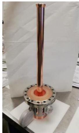
Figure 7 : Fabrication of the MYRRHA coupler designed at LPSC.
