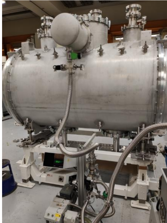
Figure 166 : Picture of the cryomodule CM1 during the final leak tightness test before the coupler issue.
