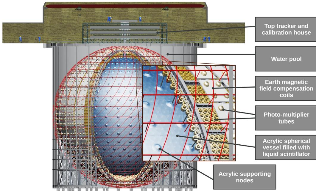
**Figure 2:** Overview of the JUNO detector with the main sub-systems.
