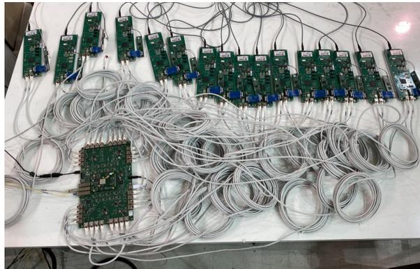
**Figure 12:** TT Electronics validation test of one CB connected to 16 ROB + FEB pairs.
