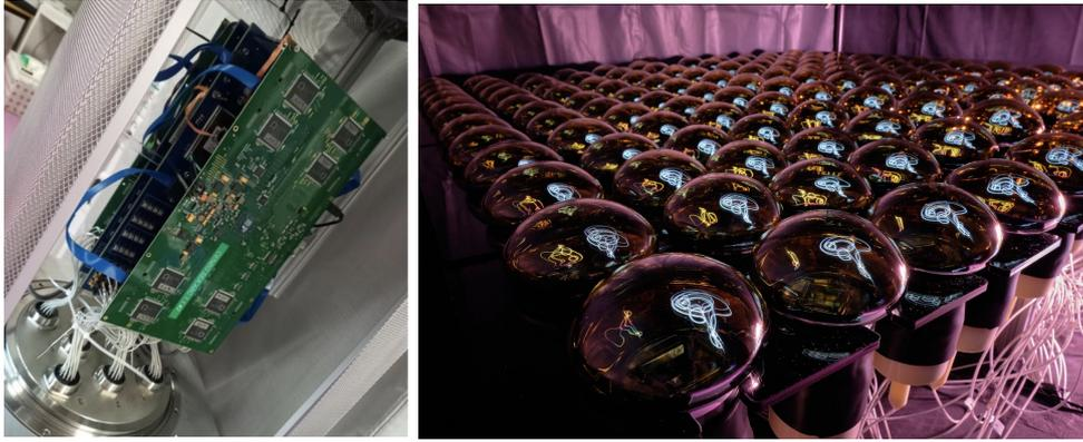
**Figure 8:** Combined test installed at CENBG, with the ABC, HV splitter and GCU boards (left) and the connected 128 SPMTs in the dark room (right).
