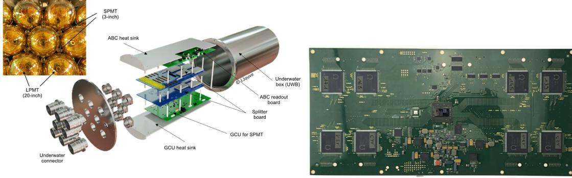
**Figure 7:** Left: Exploded view of the SPMT underwater box with the housed front-end electronics, high voltage and global control unit boards. Each connector is linked to 16 SPMTs for a total of 128 SPMTs per box. On the top left side, a picture from one of the test-bench shows the SPMT position in the space between LPMT. Right: A picture of the ABC (v1.2).
