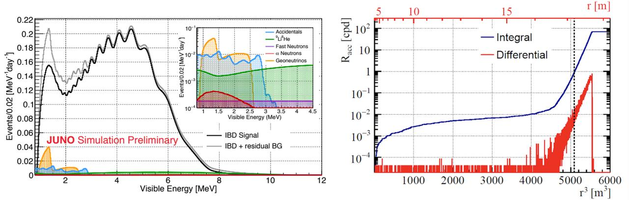
**Figure 5:** Left: Impact of the radiogenic background on the expected energy spectrum. Right: The differential (red) and integral (blue) distributions of the accidental rate as a function of the CD radius with the default selection cuts. The fiducial volume radius cut at 17.2 m is indicated as the dashed line.
