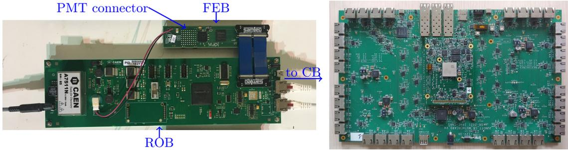
**Figure 11:** Final version of the FEB (left top), the ROB (left bottom), and of the CB (right).
