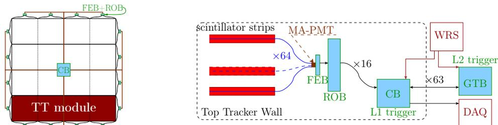
**Figure 10:** Left: Drawing of a TT wall, with one of the 8 TT modules highlighted. Right: Schematics of the TT electronics chain.
