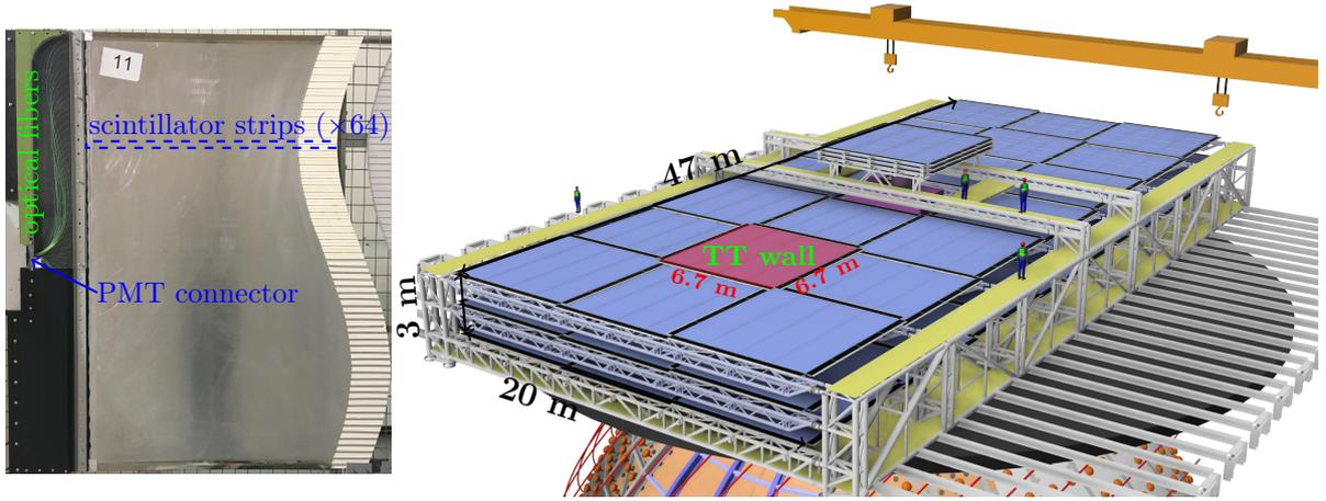
**Figure 9:** Left: Cut TT module. Right: The JUNO Top Tracker with a TT wall highlighted. From [F-1].
