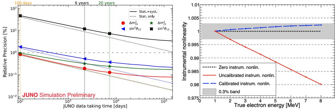
**Figure 4:** Left: Expected JUNO precision to measure various oscillation parameters as a function of data taking time. Right: Impact of the LPMT instrumental non-linearity and correction using the dual calorimetry calibration [F-2].
