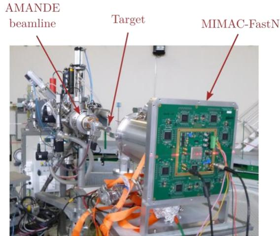
Figure 12: The MIMAC-FastN detector in front of the  $^{45}\text{Sc}$  target for low energy (8 and 27 keV) neutron fields. The chamber was filled with a low-pressure gas mixture (50% i-C<sub>4</sub>H<sub>10</sub> + 50% CHF<sub>3</sub> at 30mbar). The beam was protons at 2.912 and 2.925 MeV.
