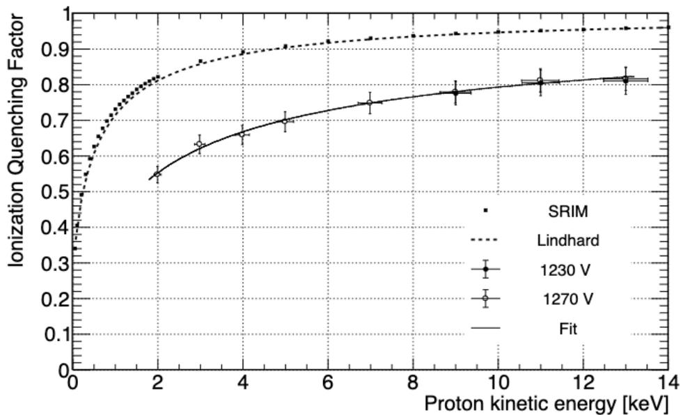
Figure 15: Ionization Quenching Factor for protons in 100 mbar of methane. The measurements at 1230 V and 1270 V are respectively presented with black dots and white dots. Comparisons with SRIM and with the Lindhard theory are also shown.
