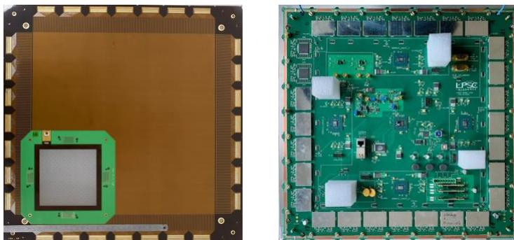
Figure 10: (Left) The new 35x35 cm<sup>2</sup> detector compared with the 10x10 cm<sup>2</sup>. (Right) The 1792 channel-electronic board.
