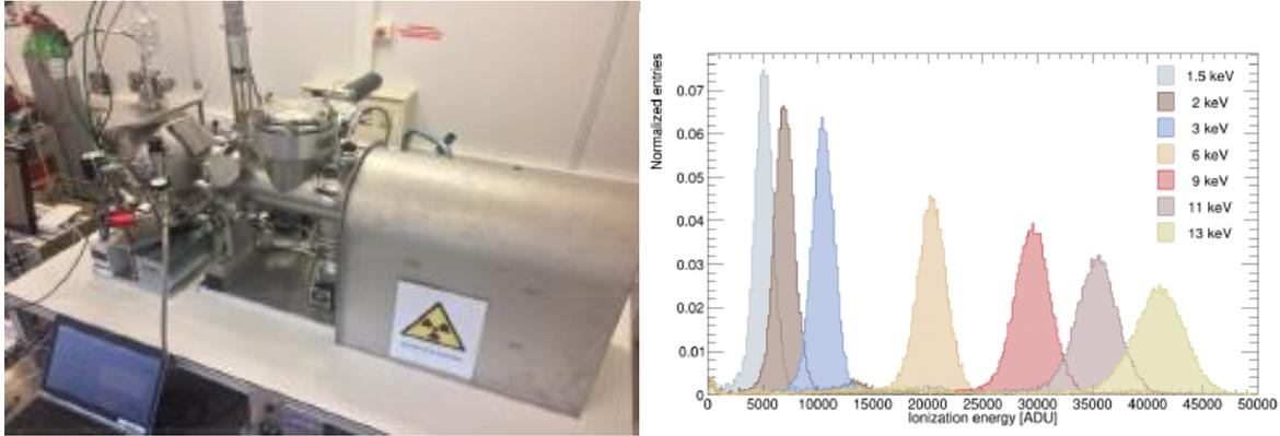
Figure 14 : Left: A picture of the experiment with Comimac on the right and the SPC on the left . Right: Complete set of energy spectra used for the calibration of the detector response. The kinetic energy is determined by the Comimac facility. The cosmic background has been subtracted but no cut is applied.
