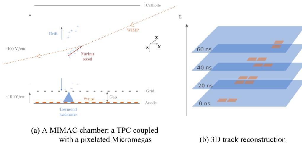
Figure 2: Schematic of the MIMAC detection principle. A WIMP induces a nuclear recoil that ionizes the gas. The primary charges drift along the electric field lines direction, i.e. along the Z-axis, towards the grid. They enter the amplification area where they produce avalanches. The signals induced on the grid and on the pixelated anode are measured every 20 ns.
