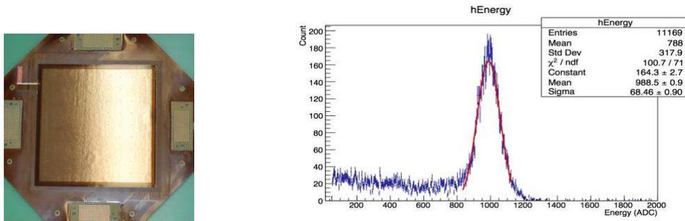
Figure 9: Left: Picture of the new low-noise micromegas bulk 10x10 cm<sup>2</sup>. Right: The <sup>55</sup>Fe- X-ray at 5,96 keV spectrum of the new detector in our MIMAC gas mixture.
