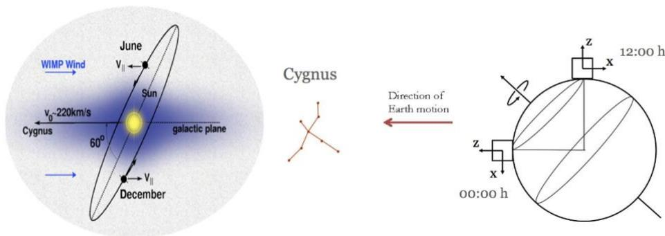
Figure 1: (Left) Scheme showing our solar system movement with respect to the galactic center and the elliptical orbit of the Earth around the Sun. The WIMP wind direction produced by the relative motion is indicated. (Right) A drawing showing how the Earth's rotation changes the orientation of the WIMP direction.
