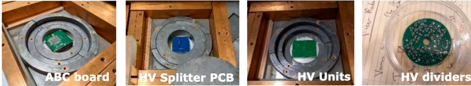
SPMT contributions: PMT+ HV divider: 66%, UWB: 21%, Potting: 13% (150 mHz in fiducial volume, <300 mHz requirement)
