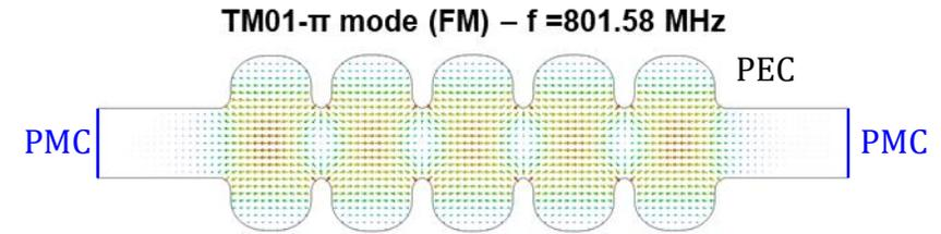
Assumption: PEC (Perfect Electric Conductor) on conducting walls (Nb) and interior domain of vacuum
