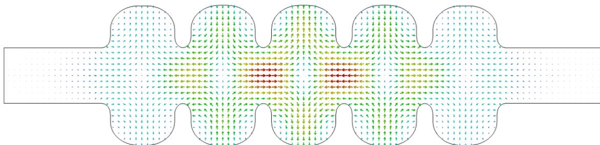
E-field - **TE111 mode** (Dipole HOM) –  $f = 933.53$  MHz
