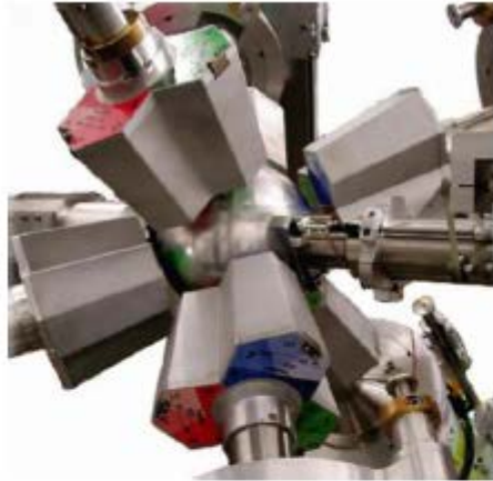
MINIBALL triple-clusters with 6 and 12 fold segmentation
