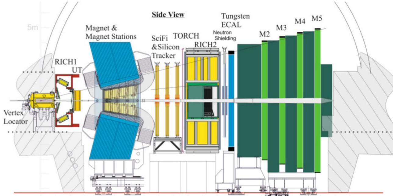
Same spectrometer footprint, innovative technology for detector and data processing
