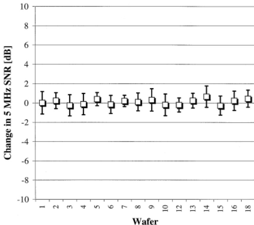
Fig. 5. Change in 5 MHz SNR for ADCs exposed to  $10^{12}$  p/cm<sup>2</sup> as a function of wafer number. The open squares represent the average of the ADCs irradiated, and the error bars the RMS.
