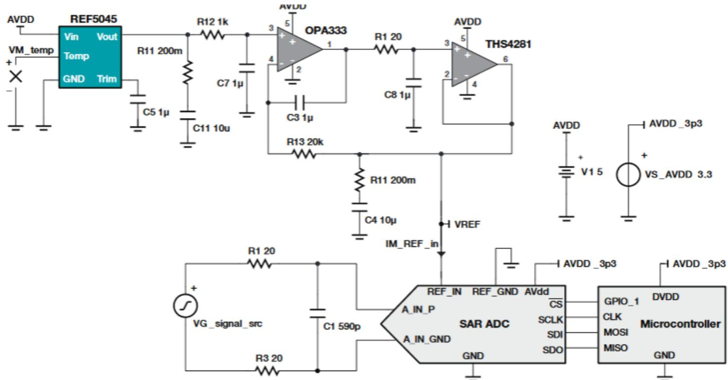
Figure 12. Schematic of a data-acquisition system with a reference buffer.
