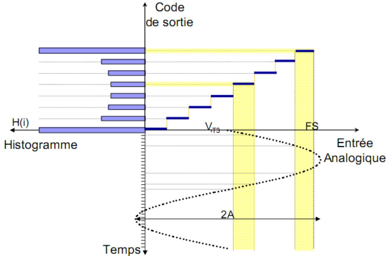
$$H^{\text{réf}}(i) = \frac{N_T}{\pi} \left( \arcsin \left[ \left( \frac{2i - 2^n}{2^n} \right) \cdot \frac{PE}{A_{\text{in}}} \right] - \arcsin \left[ \left( \frac{2i - 2^n - 2}{2^n} \right) \cdot \frac{PE}{A_{\text{in}}} \right] \right)$$
