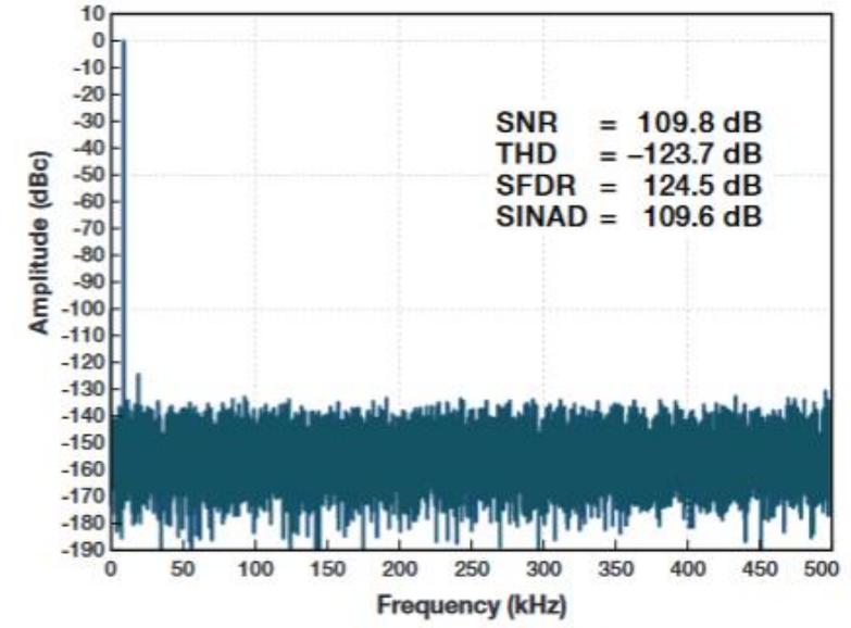
Figure 17. Key AC performance metrics and FFT for a system with the REF6045.
