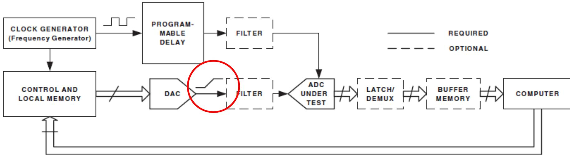
Figure 4—Setup for arbitrary signal testing
