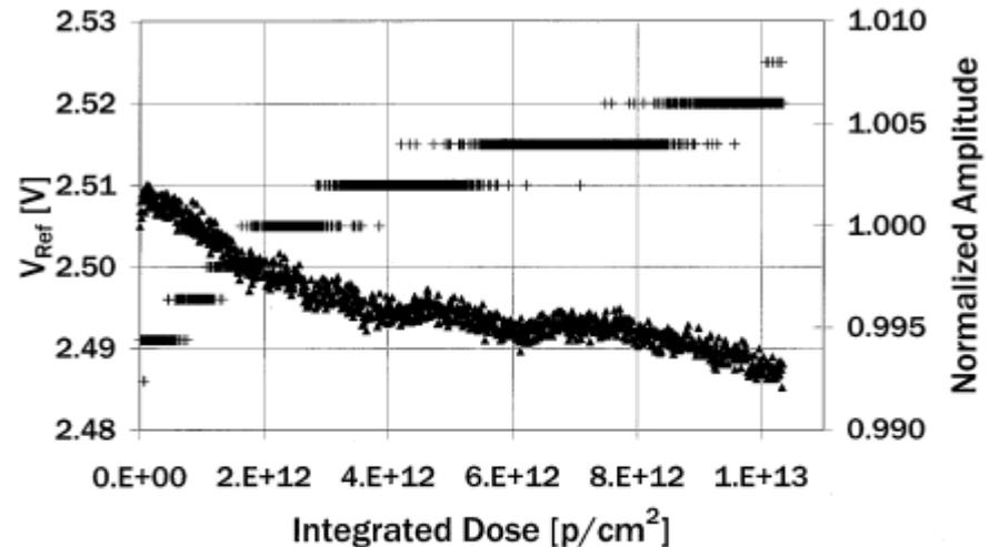
Fig. 7. Amplitude and voltage reference change during irradiation. The crosses indicate the measured value of the ADC voltage reference on the left-hand scale, and the triangles indicate the normalized change in amplitude for a 5 MHz full-scale sine wave on the right-hand scale.
