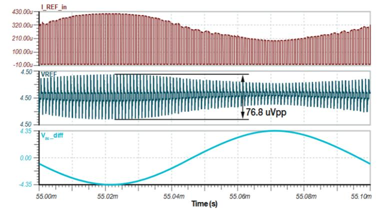
Figure 16. Simulation results for a system with the REF6045.
