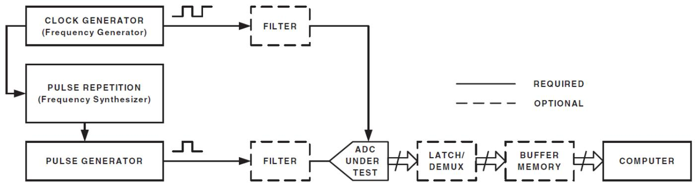
Figure 5—Setup for pulse and step signal tests
