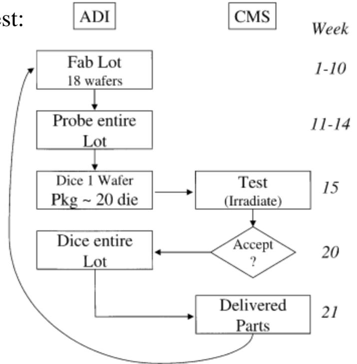
Fig. 1. ADC process flow for CMS.
