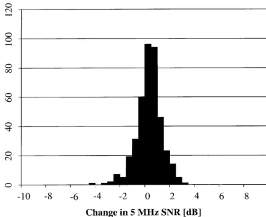
Fig. 6. Change in 5 MHz SNR for all ADCs exposed to  $10^{12}$  p/cm<sup>2</sup>, i.e. a histogram of the data in Fig. 5.
