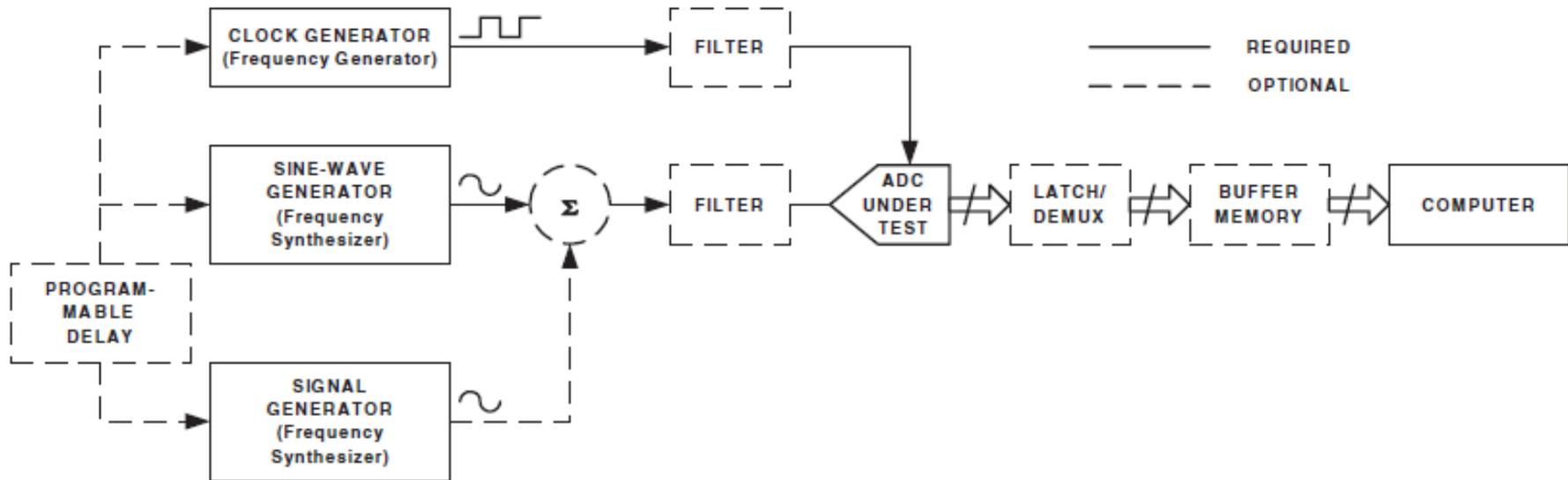
Figure 3—Setup for sine wave testing
