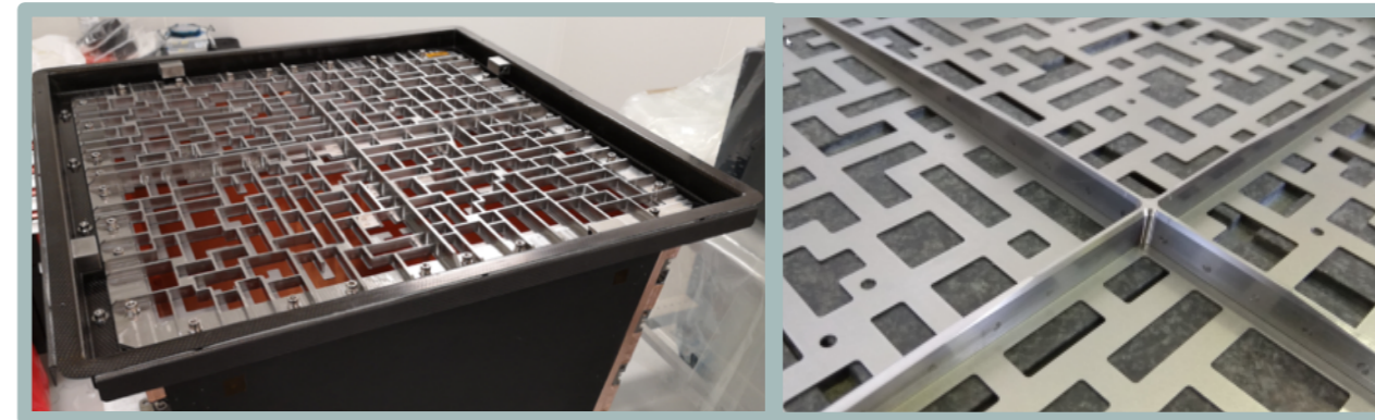
Coded mask of ECLAIRs (QM)
