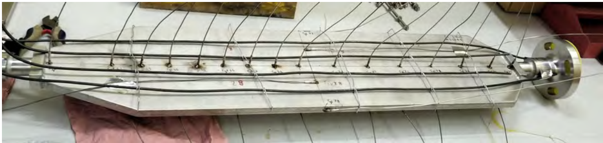
Positioning of the electric heaters and the thermocouples on the bottom wall of the flat channel.
