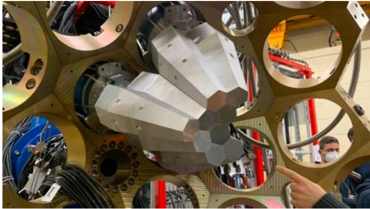
First 3 detectors mounted 400 \mu m between 2 detectors
