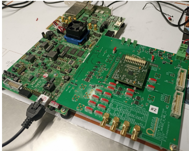
Figure 19: Test board used at OMEGA, LLR and IRFU to perform all the HKROC tests. The ASIC is mounted on a mezzanine board, itself mounted on a mother board connected to a KCU test board.
