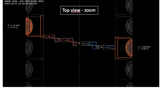
Figure 8: Double-beta candidate observed by the SuperNEMO Demonstrator (April 10th 2025).
