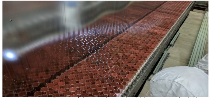
Figure 4: Some of the tracker's 15,000 wires and 4068 copper cathode rings comprising the 2034 Geiger cells.
