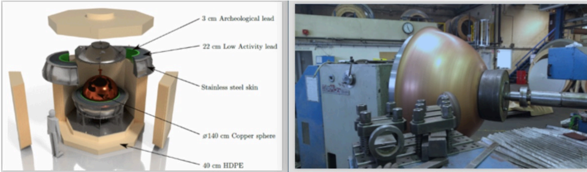
FIGURE 4 – Exploded view of the detector to be installed at SNOLAB (left) and picture of the detector construction (right).
