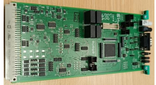
Figure 16 – Prototype of the pulser board.
