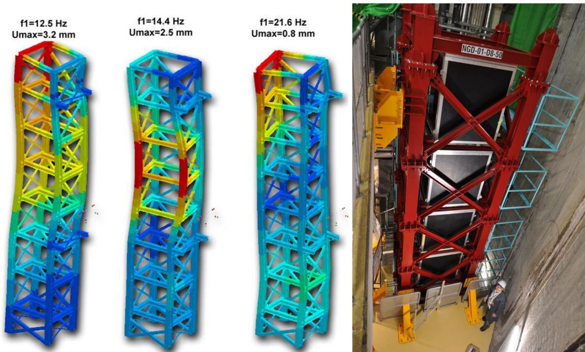
Figure 8: Left : the INGRID detector has been designed at LLR, taking into account the constraints in case of severe earthquakes. Right : the LLR engineer responsible for the project, during the construction phase.
