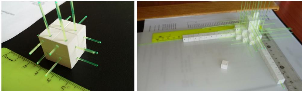
Figure 22: Picture of a small Super-FGD prototype . Several cubes of extruded plastic scintillator with three fibers inserted in the three holes are assembled. The size of each cube is  $1 \times 1 \times 1 \text{ cm}^3$ .
