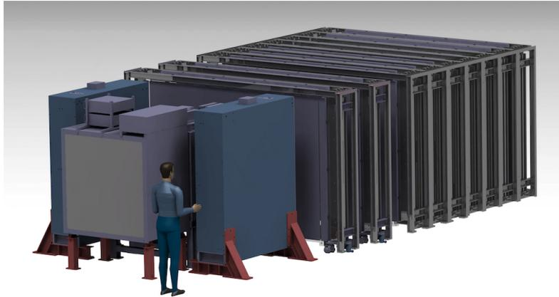
Figure 15: Schematic view of the entire set of detectors for the  $4\pi$  measurement of the WAGASCI experiment.
