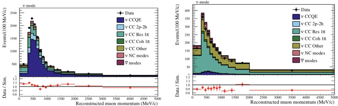
Figure 4: Momentum distribution of outgoing muons for  $\nu_\mu$  CC- $0\pi^+$  (left) and CC- $1\pi^+$  (right) samples at ND280.
