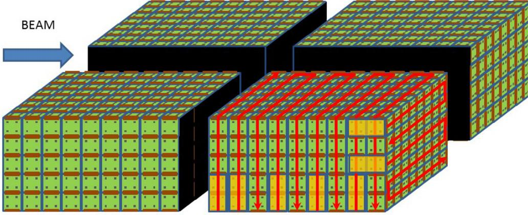
Figure 24: Schematic view of the proposed arrangement for the very front-end boards. Each quarter of the detector is read out on the top and external side panels. For each quadrant, the 7 chains of  $\sim 20$  boards are connected to 7 DIF boards (represented in yellow on the lower right quadrant), which are in turn connected to one GDCC board (located outside of the magnet) by means of standard HDMI cables (not shown).
