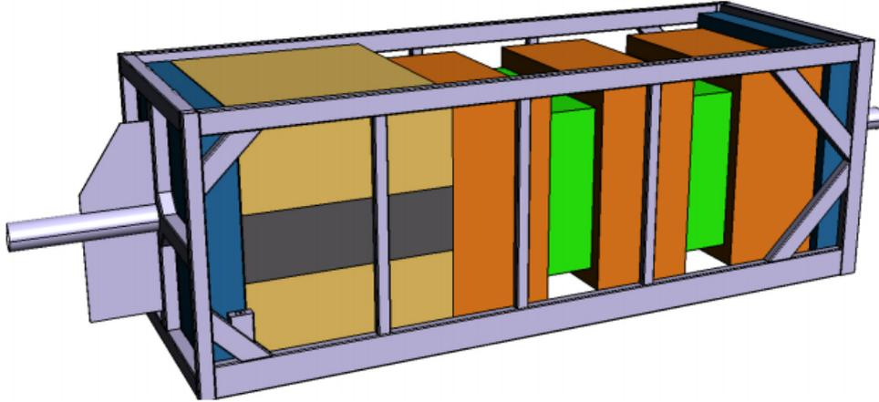
Figure 17: Sketch of the ND280 upgrade project. In the upstream part of the detector (on the left in the drawing) two horizontal TPCs with a scintillator module in the middle will be installed. In the downstream part, the tracker system composed by three TPCs (orange) and the two FGDs (green) will remain unchanged.
