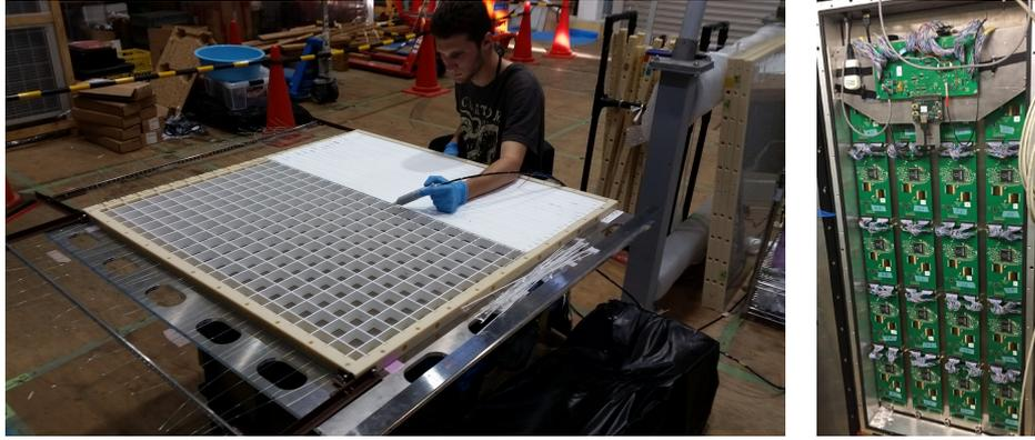
Figure 14: Left panel shows the assembly of the 3D scintillator grid. Right panel shows the DAQ chain developed at LLR for MPPC readout.
