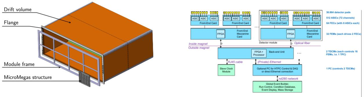
Figure 25: Left: Schematic view of the High-Angle TPC. Right: architecture of the readout system of the TPC.
