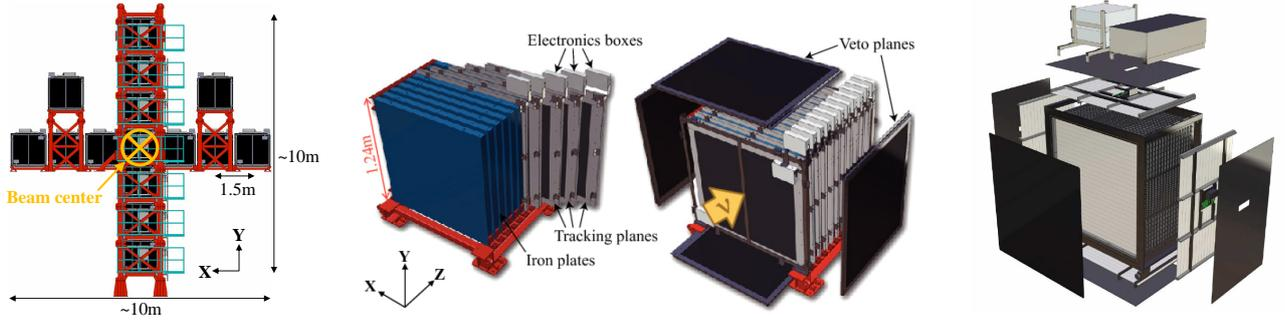
Figure 2: Schematic views of the INGRID detector (left) and of the corresponding individual modules, including the Proton Module (right).
