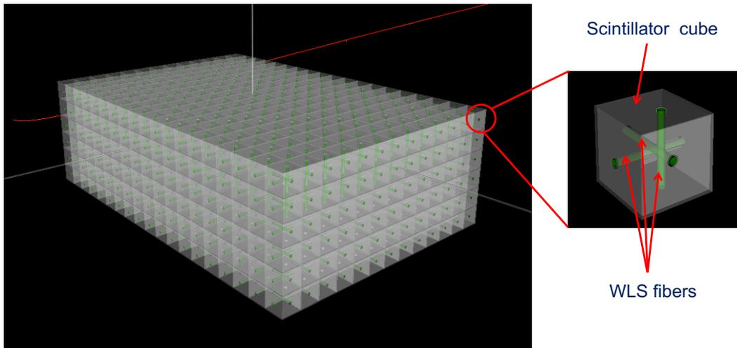
Figure 21: Schematic of the super-FGD structure.
