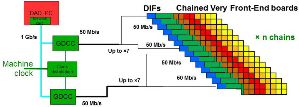
Figure 23: Schematic view of the readout and DAQ system developed for the ultra-granular calorimetry at the future International Linear Collider (adapted from [52]). For the proposed Super-FGD detector, the original silicon slabs will be replaced by chains of about 20 boards hosting 4 SPIROC(2E) chips, each chain corresponding to the readout of  $\sim 3000$  MPPCs.
