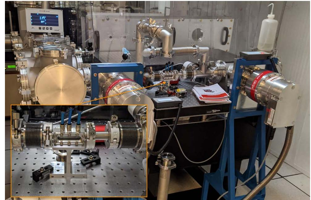
View of the plasma test bench under commissioning with long testing gas cell from Esculap project (*N. Delerue, K. Wang, S. Jenzer, et al.*)<sup>3</sup>
