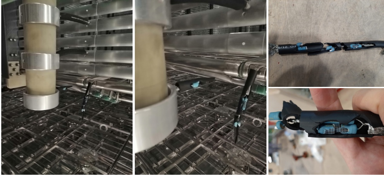
FIG. 10: Photos of the connection between the cathode and the HV extender made of a resistor chain. The blown resistors are visible inside the partially exploded shrinkable tube. The failure is most likely due to a temporary too high voltage difference between the cathode and the extender.
