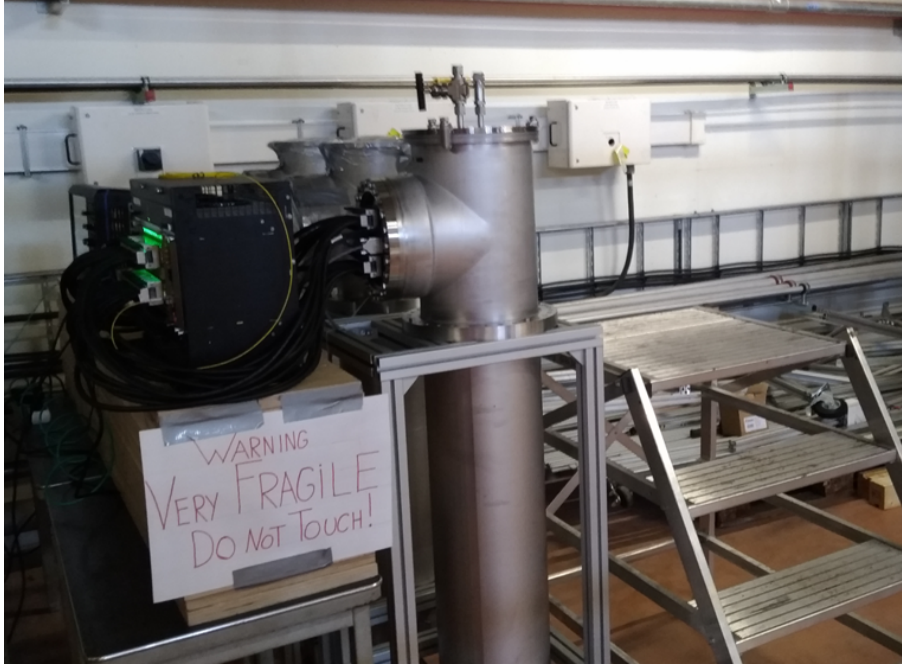
FIG. 25: Integration test of the elements of the top-drift electronics charge readout chain performed at CERN Neutrino Platform in July 2021.
