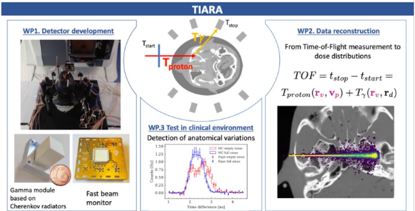
**Figure 4.1:** Left: TIARA prototype. One of the gamma modules and the beam monitor are shown in the insets. Centre: Detection principle (top) and example of TOF distributions obtained with TIARA (bottom). Right: PGTI reconstruction equation and expected output of the reconstruction algorithm.
