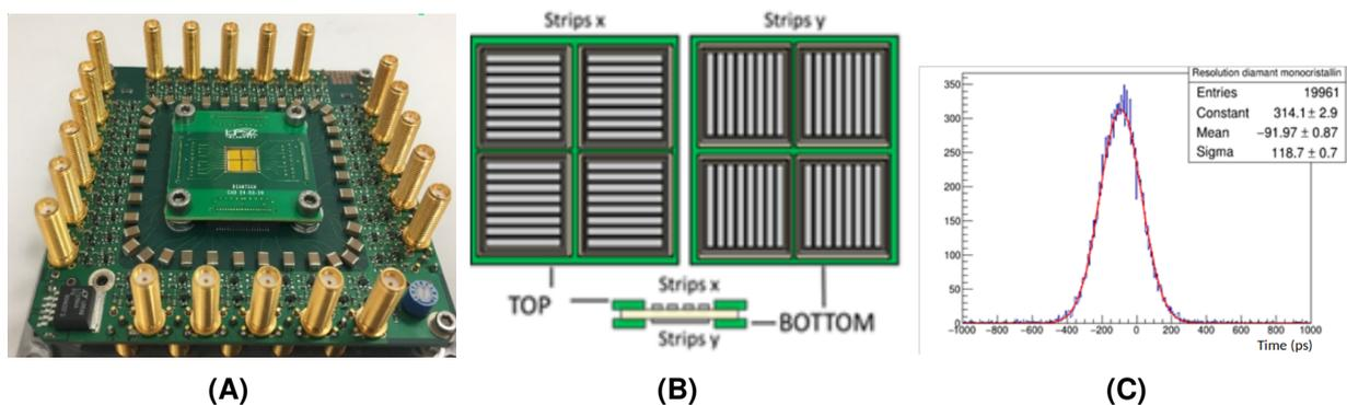
**Figure 4.5:** The Diamond beam hodoscope for on-line monitoring of the hadrontherapy (A), the stripped diamond detector mounted on its FE electronic board that consists in fast preamplifiers, details of the diamond metallisation (B) and time measurement (C) operated on the MEDICYC beamline at Centre Antoine Lacassagne that demonstrates a time resolution of less than 100 ps on a (x,y) couple of orthogonal strips crossed by a 70 MeV proton beam.
