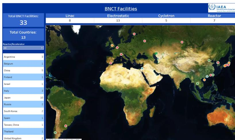
**Figure 3.3:** Visualization of the IAEA BNCT database showing the distribution of operational research reactors and the planned and operational accelerator based neutron facilities involved in BNCT. Colour code: red = electrostatic; orange = cyclotron; cyan = linac; green = reactor [IAEA, 2023].
