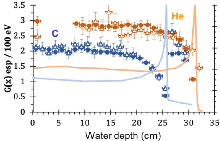
**Figure 2.9:** Radiolytic yields of  $\text{HO}\cdot$  (left) and  $e_{\text{aq}}^-$  (right) along the track of 400 MeV/u C and 230 MeV/u He ions, measured for a scavenging time of 74 ns.
