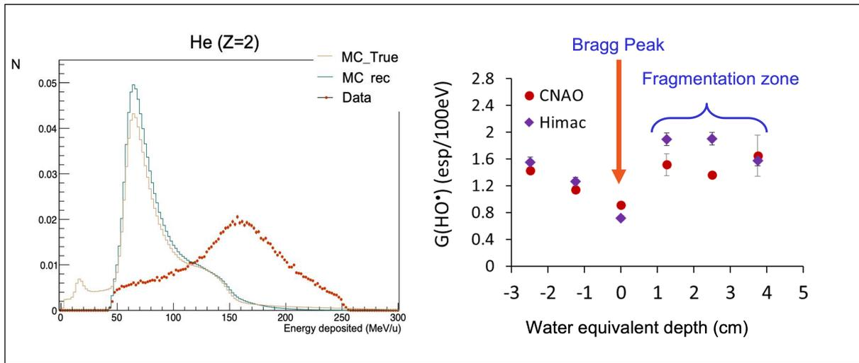
**Figure 2.8:** Left: Comparison between simulated (green line) and measured (red dots) energy distributions of Z=2 produced by a 400 MeV/u carbon ion beam interacting by 23-cm RW3 phantom. Right: Evolution of the number of HO• radicals formed per ion ( $N(\text{HO}^\bullet)/\text{ion}$ ) with the depth traversed by C ions, performed with 400 MeV/u  $^{12}\text{C}$  ions in HIMAC and CNAO.
