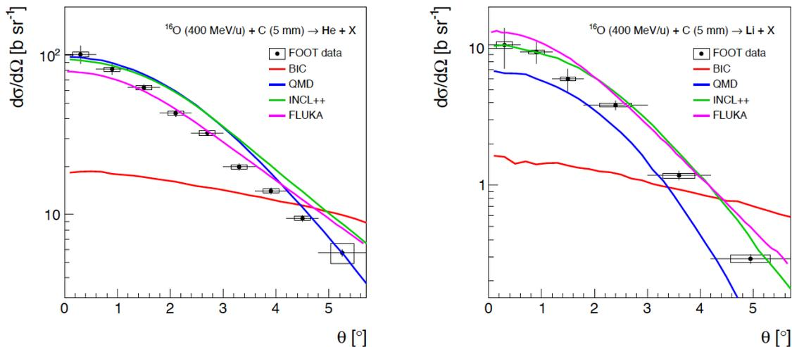
**Figure 2.7:** Angular differential cross sections for the production of He and Li fragments in the interaction process of a  $^{16}\text{O}$  beam of 400 MeV/nucleon on a graphite target together with FLUKA and GEANT4 predictions with four different models (see insert), extracted from [Ridolfi et al., 2025].
