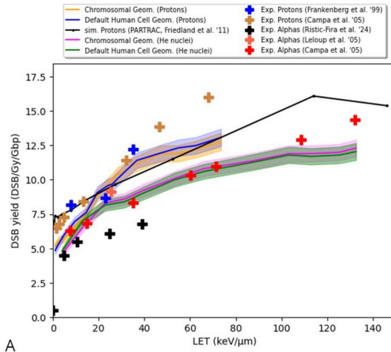
**Figure 2.5:** Quantification of Double Strand Breaks yields for several Geant4-DNA human cell models, irradiated by protons and alphas for several values of LET (lines: Geant4-DNA and PARTRAC simulations; crosses: experiments), extracted from [Chatzipapas et al., 2024]
