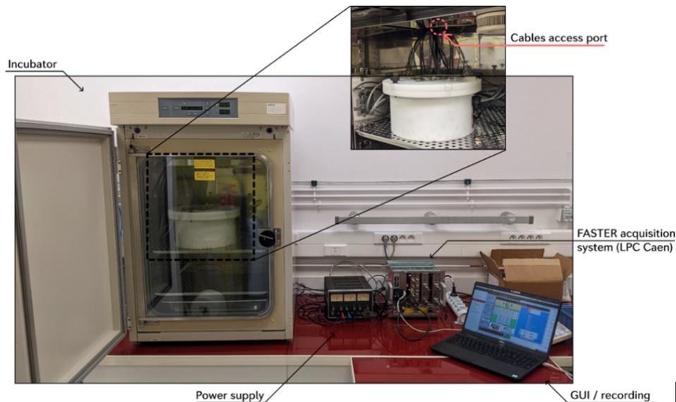
**Figure 3.6:** Experimental setup of in vitro experiments with alpha radionuclides performed at Caen with the prototype of alpha dosimeter containing four silicon detectors in a waterproof chamber.
