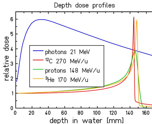
**Figure 2.1:** Dose deposition profiles of 21 MeV photons, 270 MeV/u <sup>12</sup>C ions, 170 MeV/u <sup>3</sup>He ions, and 148 MeV protons [Krämer et al., 2016].
