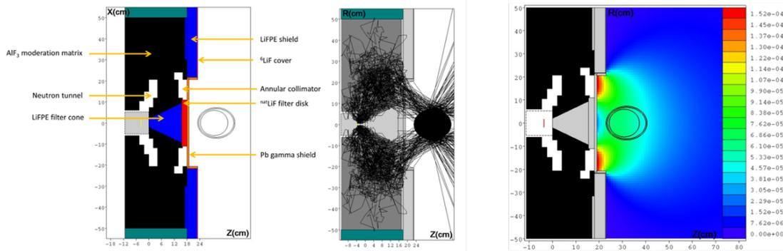
**Figure 3.9:** Example of topological optimization simulations to design a moderator for AB-BNCT facilities (based on Li target and accel. system as those of the AB-NCT installation of Helsinki) allowing to propose an optimal neutron moderation for beam intensity and spectrum [Chabod et al., 2025]
