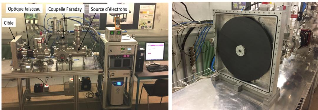
**Figure 3.8:** Left: 3 kW electron-beam test bench. Right: Graphite-based rotating target.
