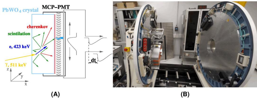
**Figure 4.13:** (A) Scheme of the ClearMind detection module. Transmission lines are read at both ends and analysed using delay lines to determine the interaction position and time ; (B) Picture of tomXgam, a double rotating mechanical test bench for experimentation in tomography.
