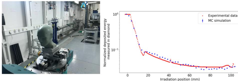
**Figure 3.11:** Left: irradiation of an anthropomorphic phantom at ESRF/ID17. Right: measurement with the diamond detector of the response to a single microbeam during a vertical translation of the phantom, compared to a GATE simulation (N. Rosuel Thesis)
