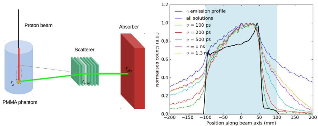
**Figure 2.6:** Simulation of prompt-gamma detection using a Compton camera with a 150 MeV proton beam incident on a PMMA cylinder (15 cm range). Top: detection scheme; bottom: comparison of profiles obtained through cone-line reconstruction with selection of solutions compatible with the measured time-of-flight [Livingstone et al., 2021]
