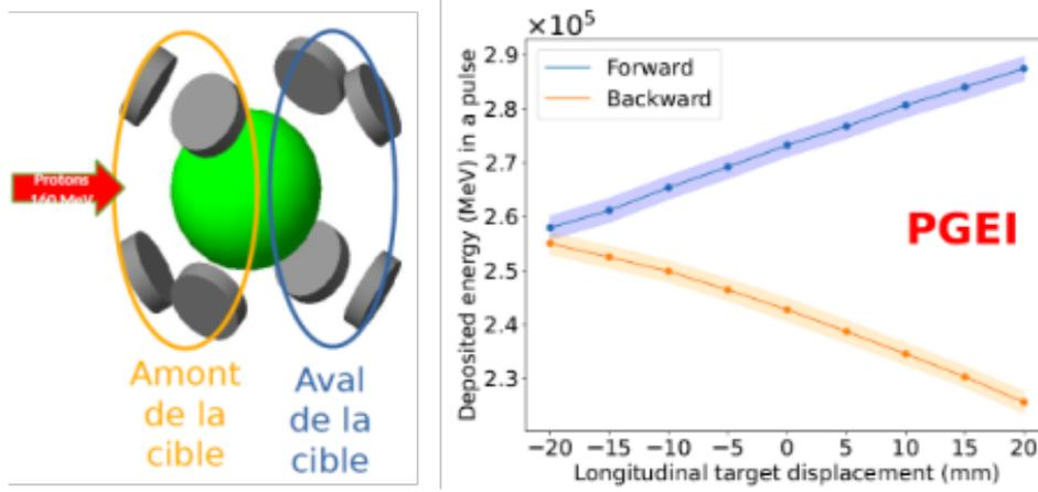
**Figure 4.2:** GATE simulations of the PGEI integral method with a 160 MeV proton beam incident on a spherical PMMA target capable of longitudinal displacement. Colored bands correspond to measurement uncertainties (at  $1\sigma$ ) for a beam spot of  $1.5 \times 10^7$  protons.
