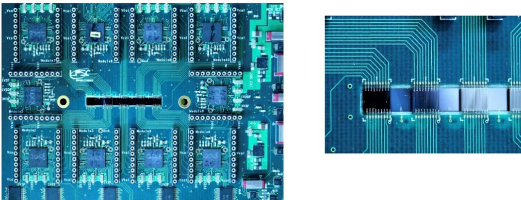
**Figure 4.7:** IDSYNCHRO detector for MRT monitoring (left: collaboration between the Detectors and Instrumentation (SDI) and Electronics Design (CAO) departments of LPSC), with an active surface (detail on the right) composed of 8 diamonds arranged in a linear array (17 micro-strips per diamond – collaboration with Institut Néel, NanoFab platform, and LPSC), read out by integrated QDC electronics developed by the Electronics Department at LPSC.
