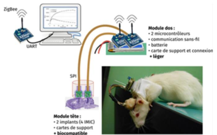
**Figure 4.12:** The detection system includes three main components: (i) a head module with probes on a mini PCB implanted stereotactically and secured with a cemented cap; (ii) a backpack module containing a microcontroller, RF system, and microbattery, connected to the head via a flexible link and held by a harness; and (iii) an acquisition module with a console and RF receiver for data transmission.
