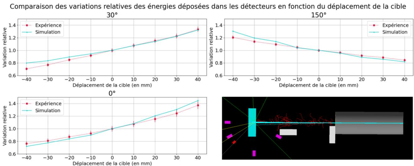
**Figure 4.4:** PGEI yields measured for proton beams stopped in a movable PMMA target at  $\sim 1 \mu\text{A}$  pulse-current, for 3 observation angles ( $0^\circ$ =forward direction). Comparison with GATE simulations (illustrated bottom right).
