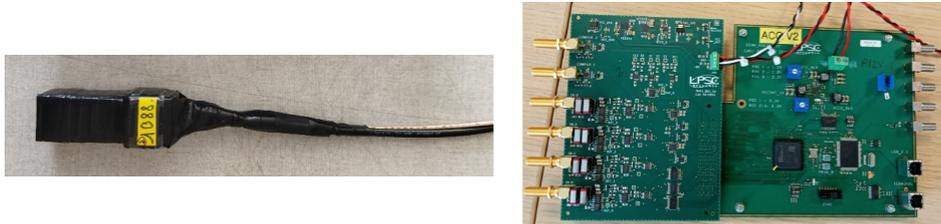
**Figure 4.3:** Left:  $2.5 \times 2.5 \times 5 \text{ cm}^3$   $\text{PbWO}_4$  scintillator coupled to PMT; right: 4-channel acquisition board.
