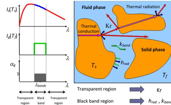
Thermal Radiation model for the salt
