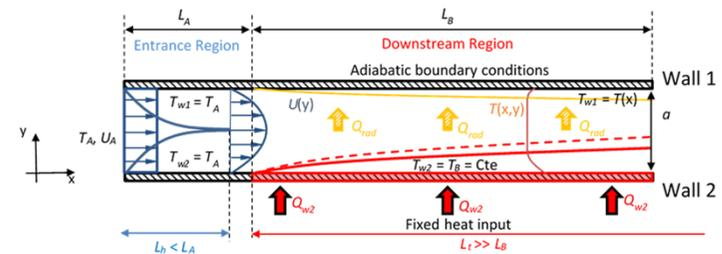
Flat Channel working principle
